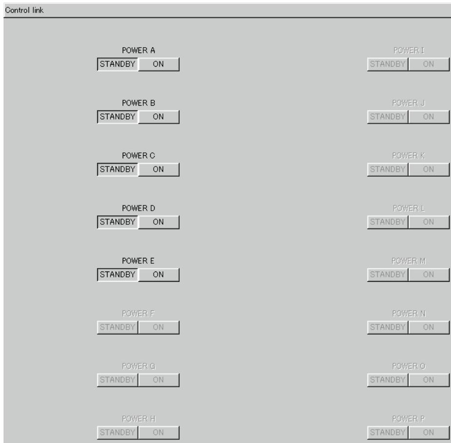
The STANDBY and ON buttons are unavailable when no power amplifiers are in a group or when the group is disabled. When a group is enabled, you can click the STANDBY button to simultaneously set all power amplifiers in that group to Standby mode. When an ON button is clicked, the amplifiers in that group are turned on.
