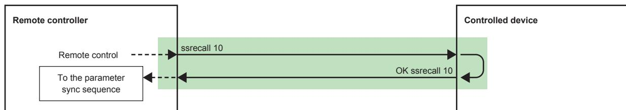
In addition, if a snapshot (preset) recall occurs internally in the controlled device (e.g. by front panel button press) or when such a request is received from another controller, the controller receives a change notification that indicates that all parameters have changed (see the next section). If this occurs, the controller needs to execute the parameter sync sequence.
