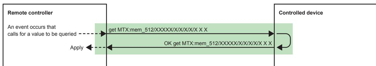
One example of using this sequence would be for refreshing the UI after boot-up or after changing tabs.
