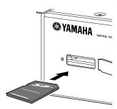
When the SD memory card has been correctly recognized, the [SD/ACT] indicator (page 9) will light. The [SD/ACT] indicator will flash while the card is being accessed.
