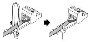
Trim off the extra portion of the cable tie as necessary.
