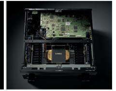
H-shaped Cross Member Frame and Symmetrical Power Amp Layout
