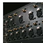
XLR balanced terminals used in pro audio equipment
